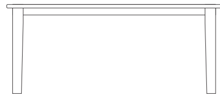
6-3 Taper Leg Table H 765mm x W 1829mm x D 915mm ALTT635
