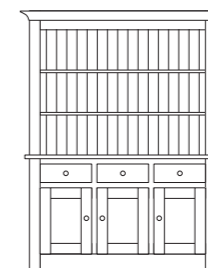
Small 3 Bay Dresser with Open Top H 1956mm x W 1550mm x D 450mm ALDA300
