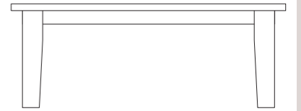
4-2 Taper Leg Coffee Table H 460mm x W 1220mm x D 610mm APOT420
