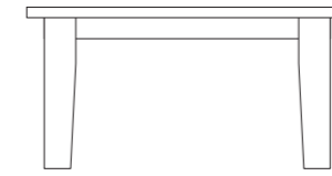
3-2 Taper Leg Coffee Table H 460mm x W 915mm x D 610mm APOT320
